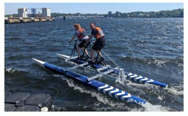
Waterbike main data: L = 6 m B = 1,1 m T = 0,5 m m = // kg V max = // knPropulsion type: Pod-Propeller
