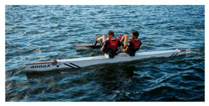
Waterbike main data: L=6 m B=2 m T=0.4 m m=70 kg Vmax=12 kn
