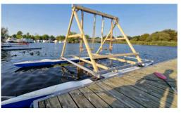
Waterbike main data: L = 3.2 m B = 0.9 m T = 0.4 m m = 120 kg Vmax = 6 kn Propulsion type: propeller
